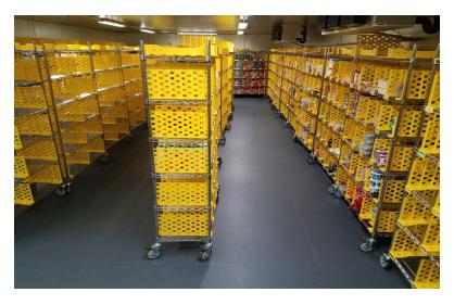
Walk-in cooler and freezer flooring can contribute to the longevity of your equipment and the safety of your staff. The wrong walk-in cooler floor can make it difficult for staff to access stored food; a challenge to move inventory in and out, and can even create serious damage to the floor beneath the cooler. Protect-All® flooring and Protect-All Rapid Weld™ make an ideal flooring system for walk-in coolers and freezers.
